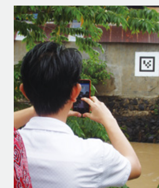
Measuring river levels using smartphones and AR technology in Manado, a city in North Sulawesi Province, Indonesia
